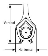
Horizontal Clearance Required Standard Duty: 4-1/4" (110 mm) Heavy Duty: 5-1/4" (135 mm)
